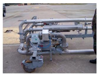
**PANTOGRAPH** with Water/Solid Sensor
