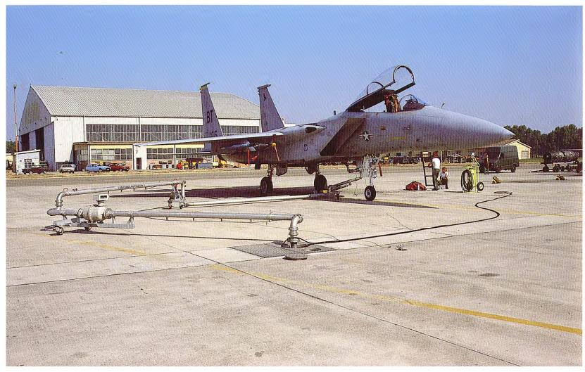
CLA-VAL-Hot refueling PANTOGRAPH with flow meter and CLA-VAL hydrant pit valve
