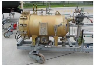
PANTOGRAPH with Filter/Water Separator
